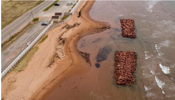
Figure 1. NbI for coastal erosion in PEI [9]. Photo credit: M. Davies, Coldwater Consulting Ltd.
